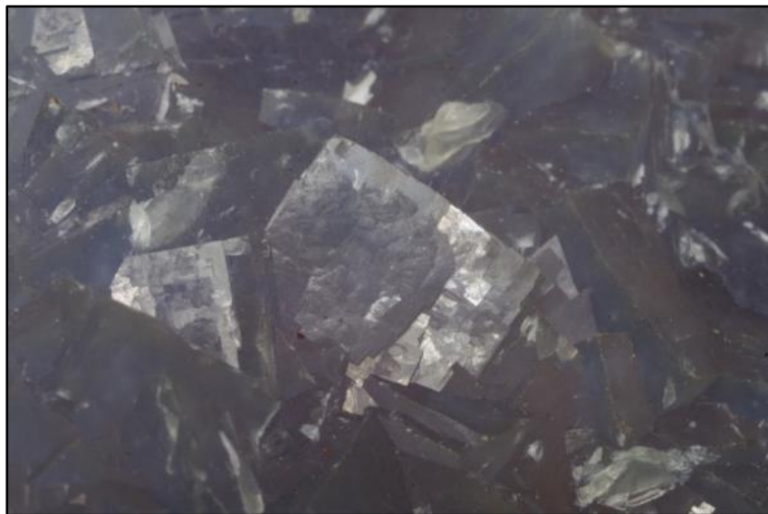
Figure 8. Macrophoto of large cube faces showing characteristic ‘tiled’ appearance. DM specimen, width of field of view 22 mm. Photo DM.
