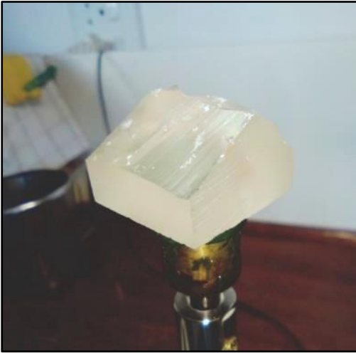
Left. Figure 3 The dopped 90 g piece of cerussite, roughly ground square
