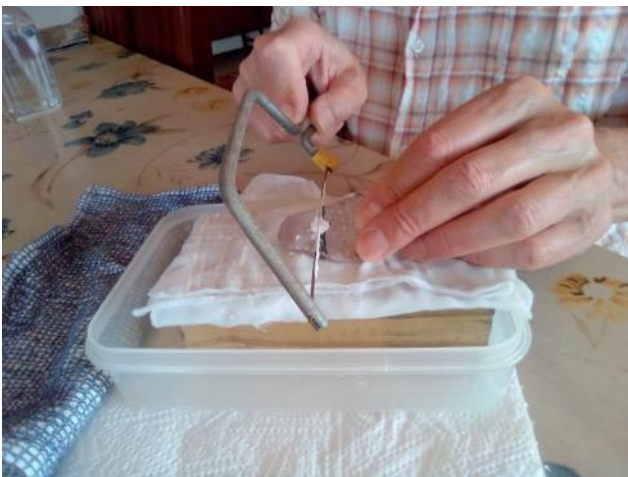
Left. Figure 1 Sawing a 119 g piece of cerussite by hand with a diamond wire saw
