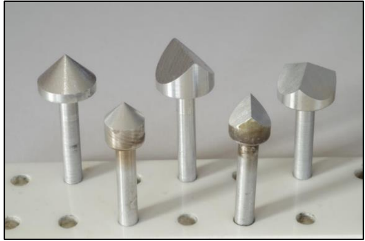
Right. Figure 4 A set of 'anti-dops' for making suitable impressions in wax for cold transfer
