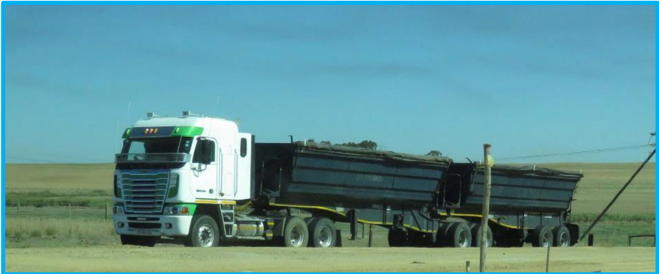
Side-Tipper Ore Transport Truck, N7
