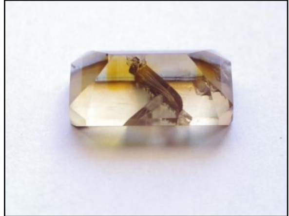
Figure 2. A 20 × 10 mm barite from Brukkaros in Namibia, with cleavage fractures caused by using a hot blade to remove excess wax after transfer – a not-to-be repeated mistake.
